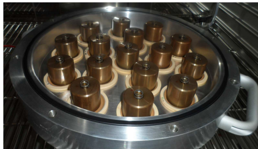
Fig.3 Photograph of the samples ready to be aged in the N 2 pressurized cell designed and built for the study before top closing, pressurization and voltage switch-on
